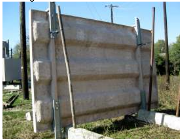
Fig. 3b: GFRC Ribs and beams on back
